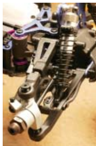
Long travel suspension is damped by high-capacity aluminum shocks (with rubber dust boots). Cast aluminum spindles are attached to the beefy aluminum steering drag link. Adjustable turnbuckles are standard.
