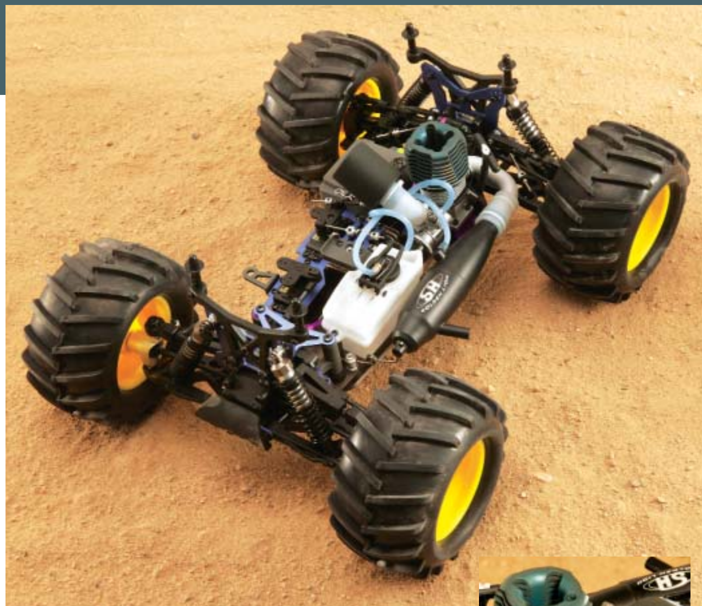
Long travel suspension is damped by high-capacity aluminum shocks (with rubber dust boots). Cast aluminum spindles are attached to the beefy aluminum steering drag link. Adjustable turnbuckles are standard.
