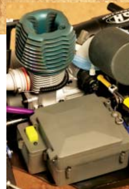
The pro version of the Rancho comes with this powerful Team Infinity Japan pull-start engine and aluminum tuned exhaust. The sealed radio box provides excellent protection for the receiver and battery. ©
